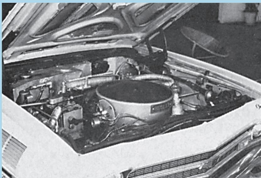
At first glance it looks like your ordinary, garden-variety Chevelle. But on closer examination the astute observer will note louvers in the hood and front fenders, cut there in order to dissipate the tremendous heat generated by the burner and the boiler. And posted on either side of the car is a neat little chrome-plated badge reading “SE 124” (Steam Engine, 124 cubic inches displacement.)
